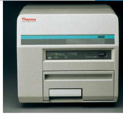
The Harshaw 3500 includes a sample drawer for a single element TLD dosimeter, a linear, programmable heating system and a cooled photomultiplier tube with associated electronics to measure the TL light output. The manually-operated Harshaw 3500 is used in medical physics, health physics, materials research, food irradiation and industrial applications.
