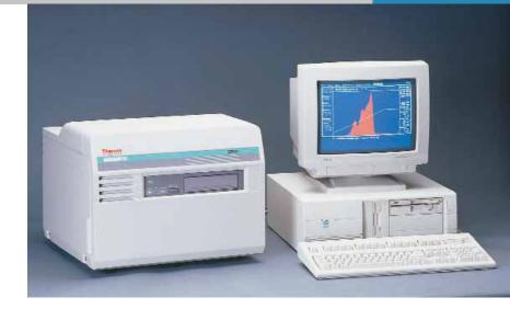
The Harshaw 5500 has a linear, programmable heating system and a cooled photomultiplier tube with associated electronics to measure the TL light output. The WinREMS Software, which runs on a separate computer, provides the user interface, the reader control and the applications software.
